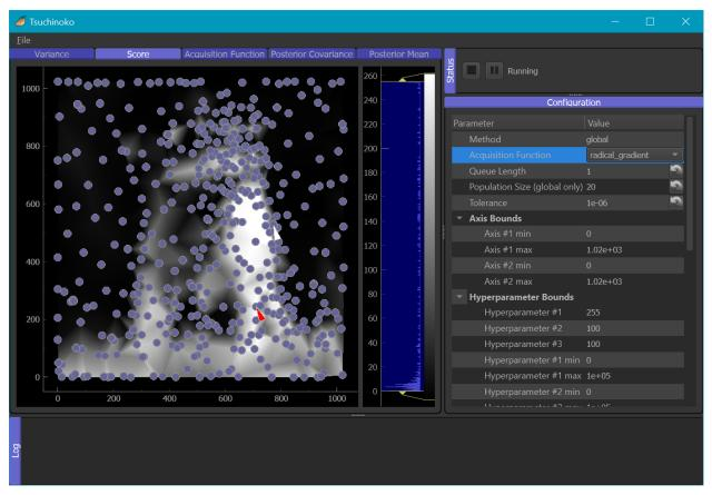
While Tsuchinoko is designed to allow custom adaptive engines to drive experiments, the gpCAM engine is a featured inclusion. This tool is based on a flexible and powerful Gaussian process regression at the core.
